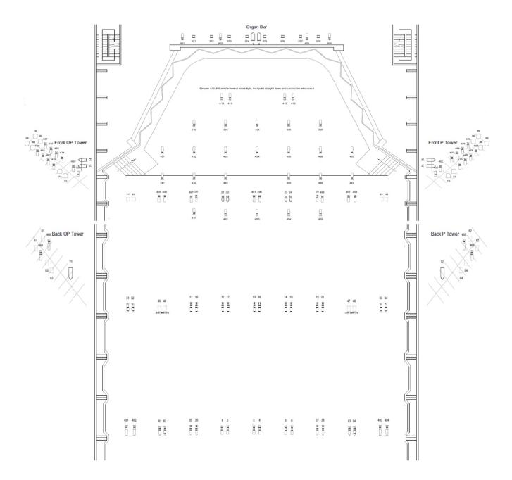
The Perth Concert Hall has approximately 200 fixtures of varying types in use within the main auditorium. We have a 50/50 mixture of conventional and LED colourful lights for front, side, back, and top stage light. Given the enormous labour cost involved, in general, fixtures are not physically moved. Wherever possible, it is preferable to work within the standard rig and refocus where applicable. Lighting gel needs to be arranged beforehand to ensure that we have the specific colours available.
