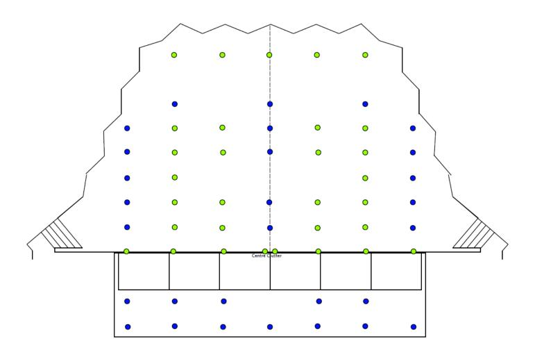
The Concert Hall has two D8+ motors permanently mounted for securing the audio line array. There is an additional four C1 motors mounted to a monorail system giving limited positions of use, for the positions that can't be covered by these motors there are an additional six C1 chain climbers.
